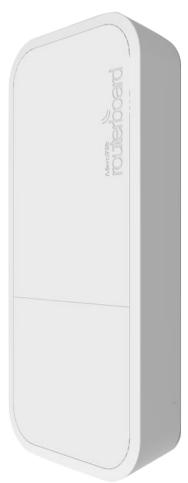
For example, when using a typical 7Ah battery, our popular wAP access point would work up to 20 hours and the LHG would work for up to 10 hours when powered only by the battery (if ambient temperature above 10C). Please note that in low ambient temperature your baterry capacity will be lower than nominal. You can refer to your battery datasheet for exact data.
